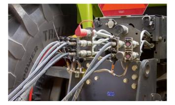
The XERION has three double-acting spool valves at the front (max. two spool valves if a front linkage is installed). Eight further double-acting spool valves are available at the rear. With quick-release couplings, you can connect and disconnect them rapidly without risk of oil leaks.
