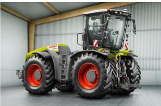
The TRAC VC has the most convenient reverse-drive system on the market. Its cab can be rotated through  $180^{\circ}$  in less than 30 seconds.
