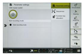
Set the parameters in the CSM overview. You can assign the function keys on the control lever as required.
